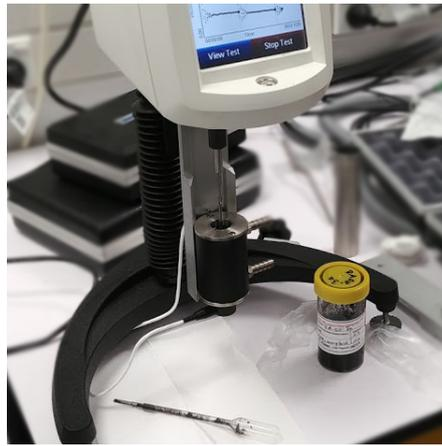
**Figure 1** Brookfield DV3T viscometer
